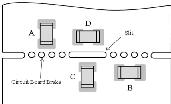
Stress strength according to the mounting position:
